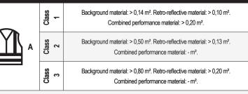
The coefficient of retro-reflection of the retro-reflective material must be class 2 to comply with EN ISO 20471 (class 1 of previous EN 471 standard has been cancelled). «X» indicates the class of the garment according to the compulsory minimum area..
